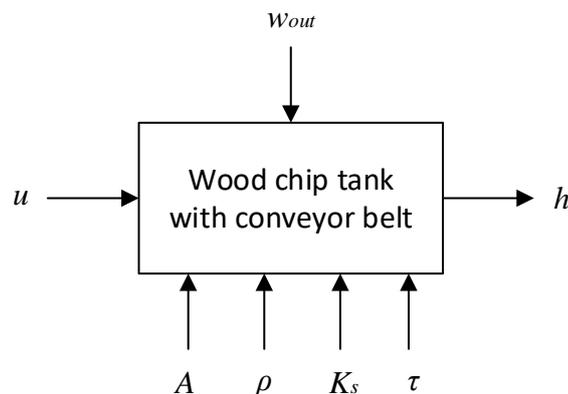
Figure 39.2: Block diagram of the wood chips tank.
