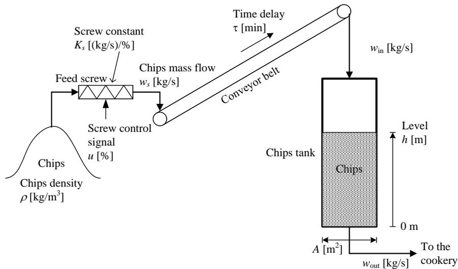
Figure 39.1: Wood chips tank.
