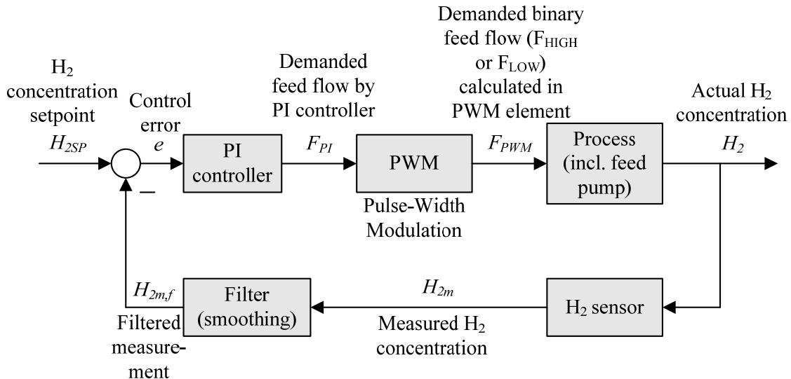
Figure 3. Block diagram of the  $H_2$  concentration feedback control system.
