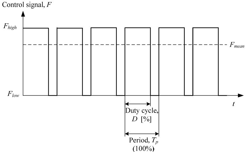
Figure 3. Pulse-Width Modulation (PWM), which is used to control the feed pump.
