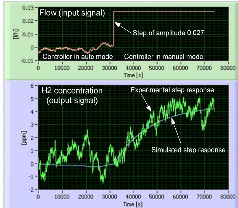
Figure 4. Response in measured (and filtered)  $\text{H}_2$  concentration due to a step change of the feed flow. Also, the simulated response with the estimated model is shown. *Deviations from the operating point are plotted.*
