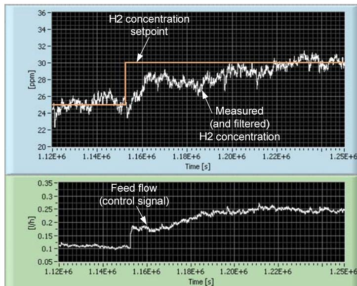
Figure 5. Responses in the  $H_2$  concentration control system.
