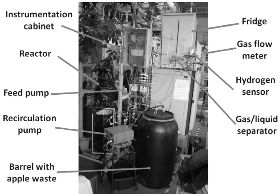
Figure 2. The biogas reactor.
