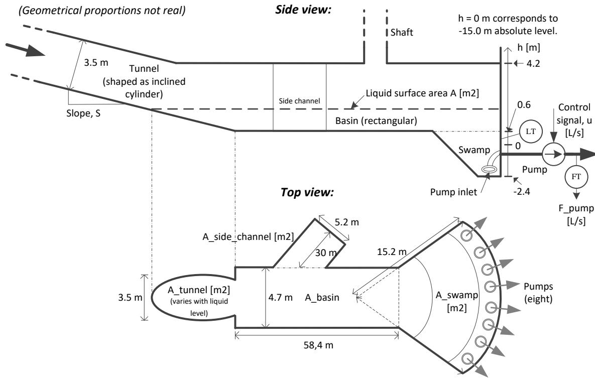
**Figure 1.** Principal design of inlet basin of VEAS WWTP.
