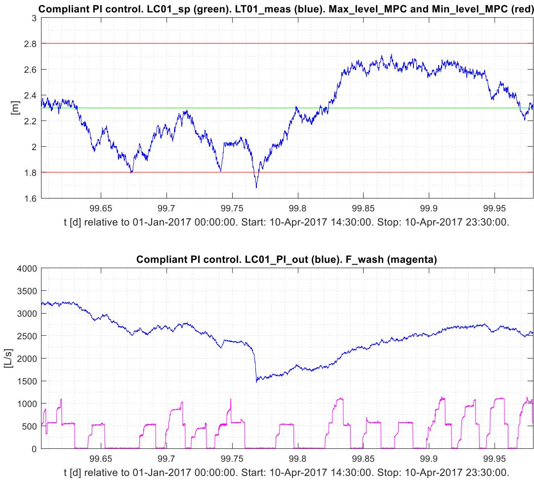
**Figure 4:** Results with PI control in Operation mode #1 (compliant level control). Time range: 9 h.
