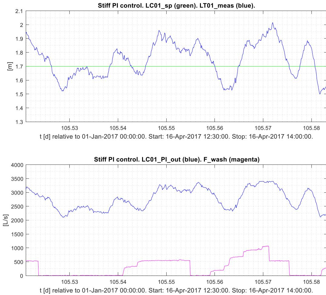
**Figure 6:** Results with PI control in Operation mode #2 (stiff level control). Time range: 1.5 h.
