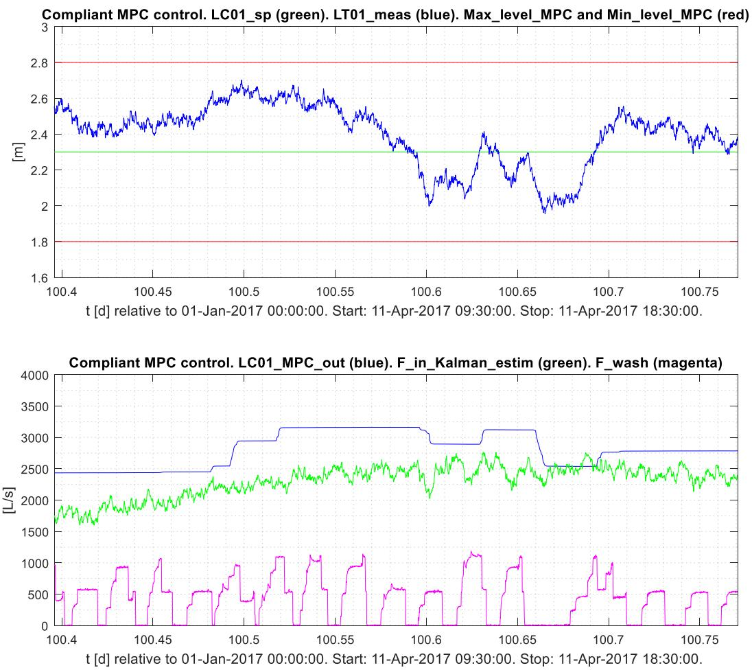
**Figure 3:** Results with MPC in Operation mode #1 (compliant level control). Time range: 9 h.
