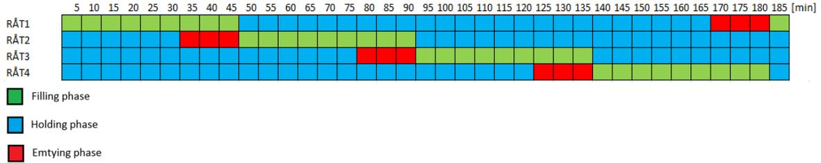
**Figure 1.** The three various phases of one cycle of operation of AD reactor
