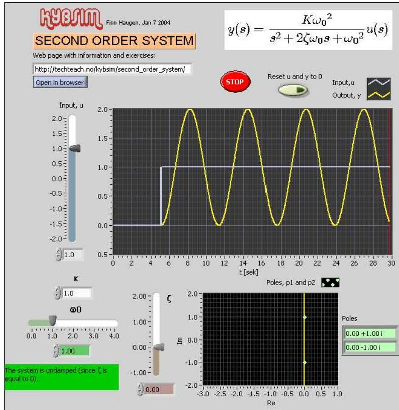
Figure 8: Step response and the poles for an example of an undamped system
