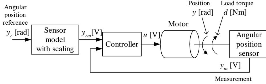
Figure 9: Feedback control system for the angular position of an electro-motor
