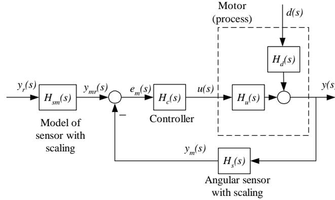
Figure 10: Transfer function based block diagram for the positional control system shown in Figure 9
