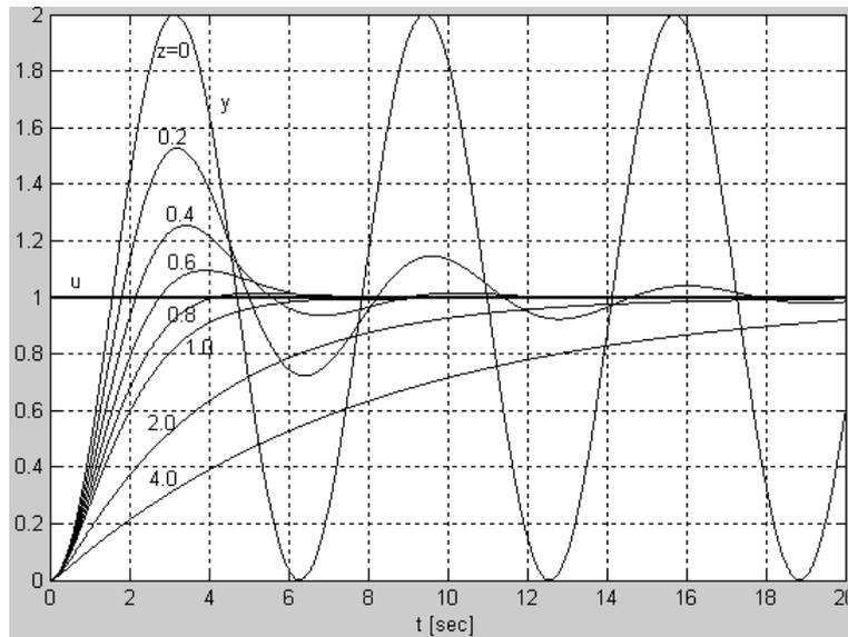
Figure 6: Step-response for various values of  $\zeta$  for second order systems
