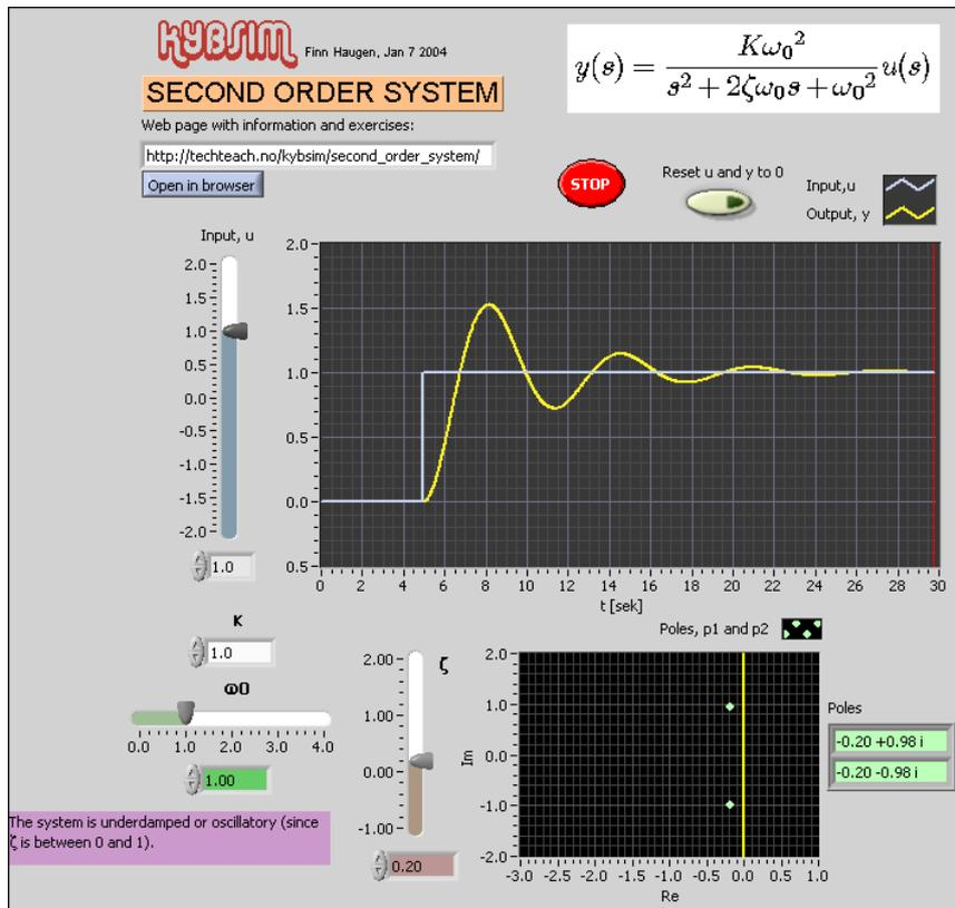
Figure 5: Step response and poles for an example of an underdamped system
