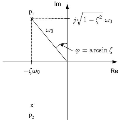
Figure 2: Pole placement for second order systems when the poles are complex conjugate. The poles are given by (13).
