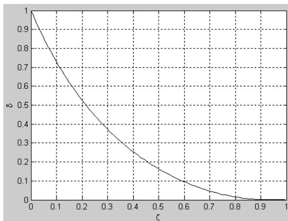
Figure 7: Overshoot factor  $\delta$  plotted as a function of the relative damping factor  $\zeta$ , cf. (19)
