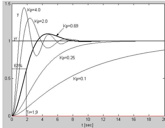
Figure 11: Simulated step responses in the angular position  $y$  (it is a step of amplitude 1 in the reference  $r$ ) for several  $K_p$ -values
