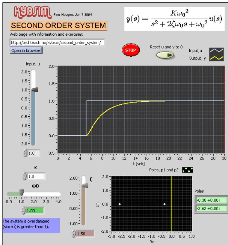
Figure 4: Step response and the poles for an example of an overdamped system
