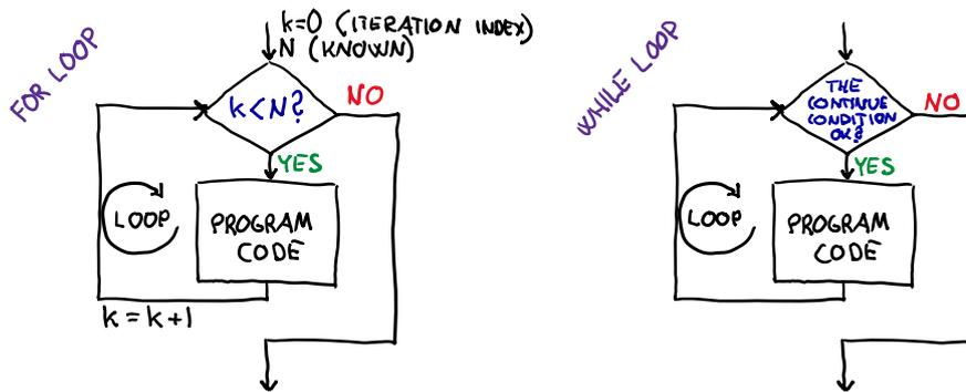
Figure 8.1: Program loop charts for for loop and while loop: Program loops are used to iterate program code execution.
