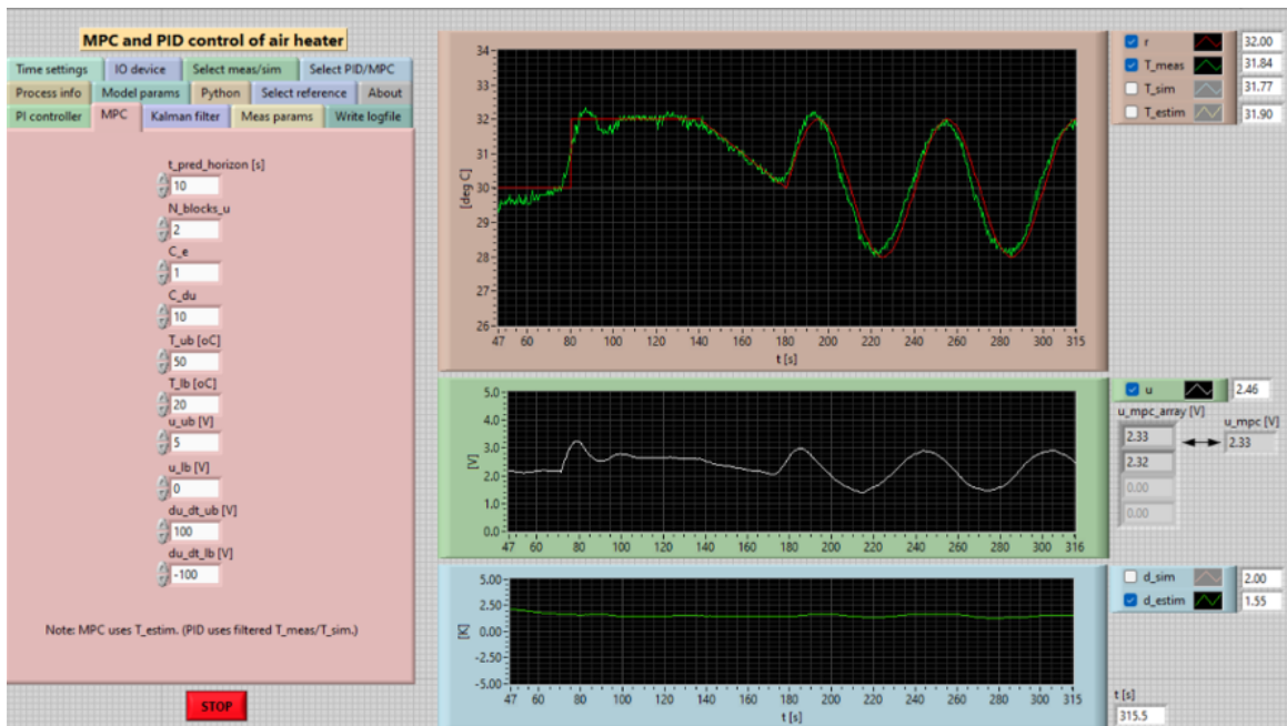
Figure 35.4: MPC control of a real air heater.
