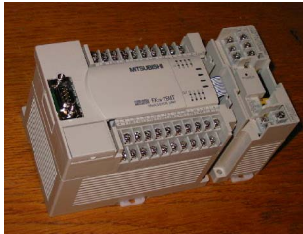
Figure 3.4: A PLC (Programmable Logical Controller). (Mitsubishi FX2N)
