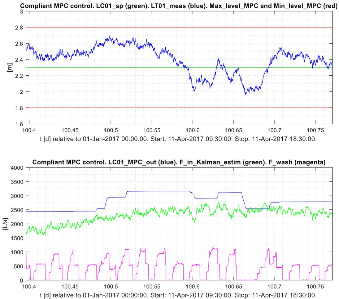
**Figure 3:** Results with MPC in Operation mode #1 (compliant level control). Time range: 9 h.
